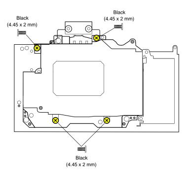
Bob's Custom Made Sony A7iii Repair Manual Screw Layout Guide - Diagram #3
